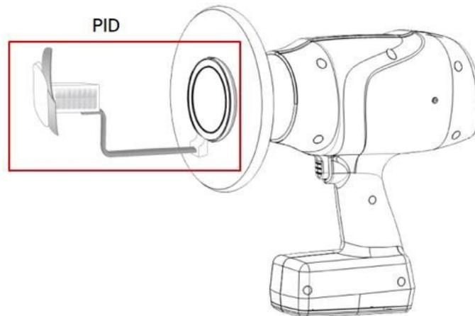
When using the PID, the exit pattern of the X-ray device should be aligned perpendicular to the target receptor as shown in the following figure.
