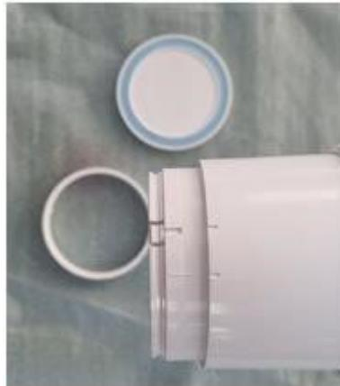
③ Fastening backscatter shield and collimator as below picture. Lock the collimator by turning as the above ① picture.
