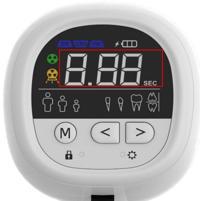
The X-ray exposure time can be set in the range of 0.02 to 0.5 sec and adjustment by 0.01 sec step.
