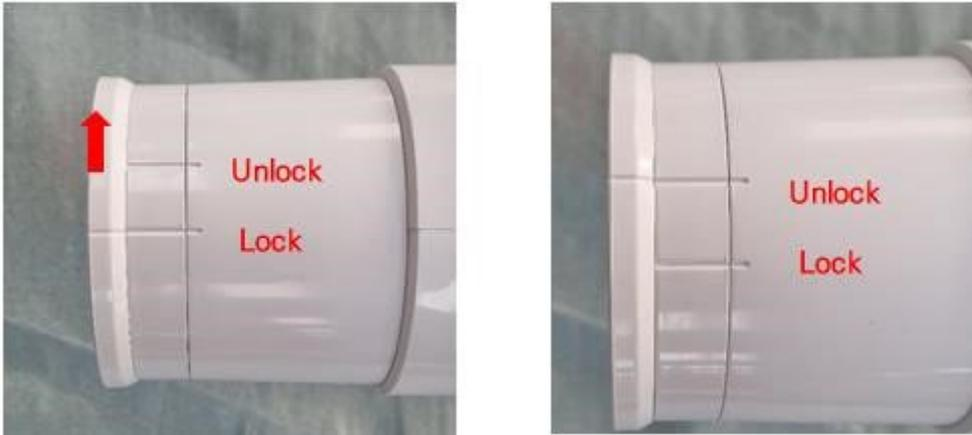
② Remove the collimator and backscatter shield ring as the below picture.
